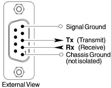
For communication with the Controller via a PC, the interface connections are illustrated in the following figures.
