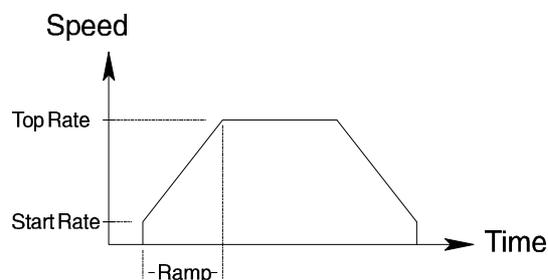
All 3 parameters must be specified in a program and can be adjusted at any point in the program. If T (Top Rate) is set to a value less than S (Start Rate), the motor will operate at the Top Rate specified by T without accelerating or decelerating.
