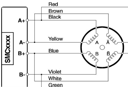
**Connection of Zebotronics motor
