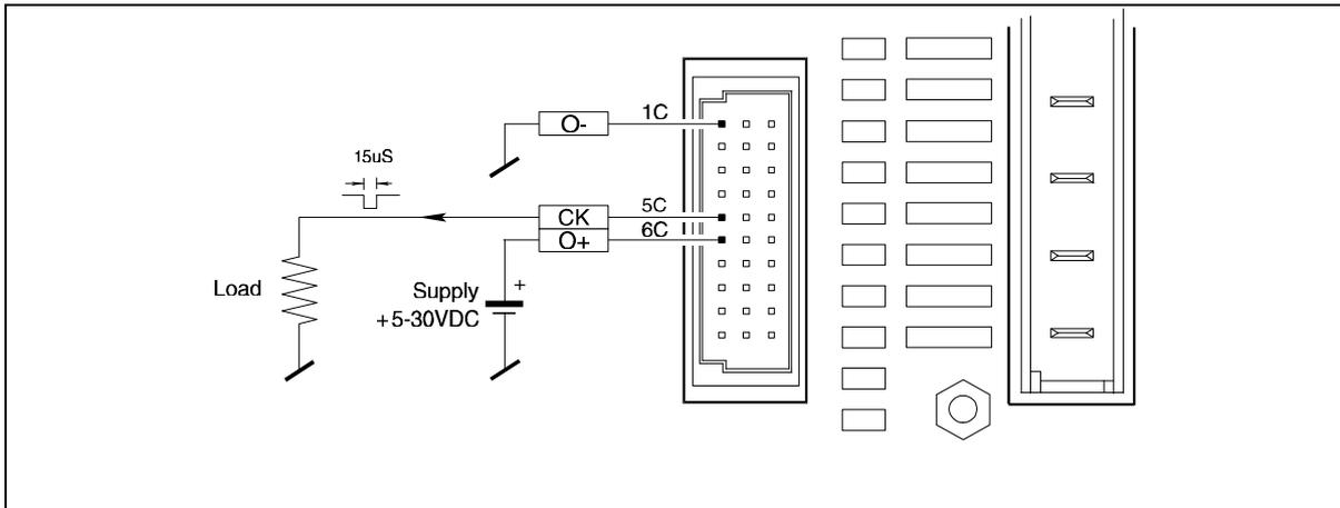
For use in motion-control systems where several step motors are operated synchronously, Controller SMC30 is equipped with a step-pulse Clock Output which outputs a voltage pulse for each motor step. The Clock Output can also be used for connection of a counter or similar equipment which is used to track motor position.
