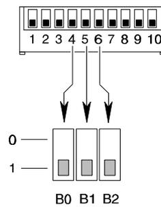
**IMPORTANT! :** If the Baud Rate setting has been changed, the Controller must be reset by switching the power off and on again for the new Baud Rate to take effect.
