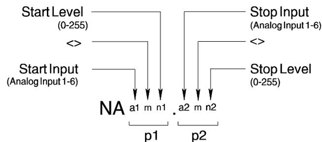
**p1:** If the start conditions are fulfilled, the motor is started. If p1 is assigned the character X, an unconditional start is defined, and the motor will start immediately the motor command is executed.
