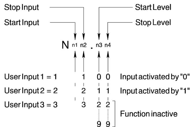
**n1:** Specifies the User Input (1-3) used to start the motor.
