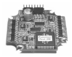
Step Motor Driver SMD73 is a miniature driver that measures only 52.4x52.4 mm and is ideal for direct mounting onto a step motor. It fits onto most types of high-torque motors, but of course can also be mounted on a surface.
